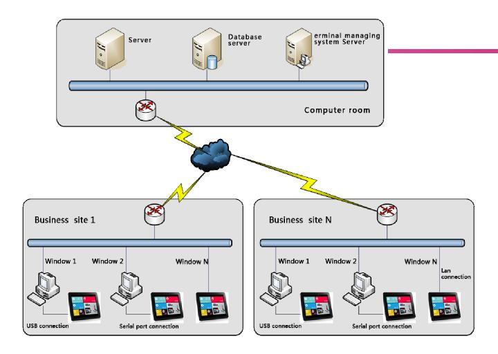
[Note:] when Wintek M8 Customer Intelligent Terminal connect to pc or client side through serial port, or when it connects to LAN directily through RJ45 interface, Wintek communication suite need to be installed.
